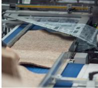
The insulative wool layer is wrapped in compostable plant-based plastic to make it 'food safe' (Photo: Planet Protector Packaging).
